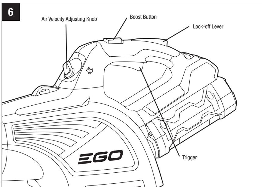
The blower is equipped with stepless speed regulation to control air speed.
